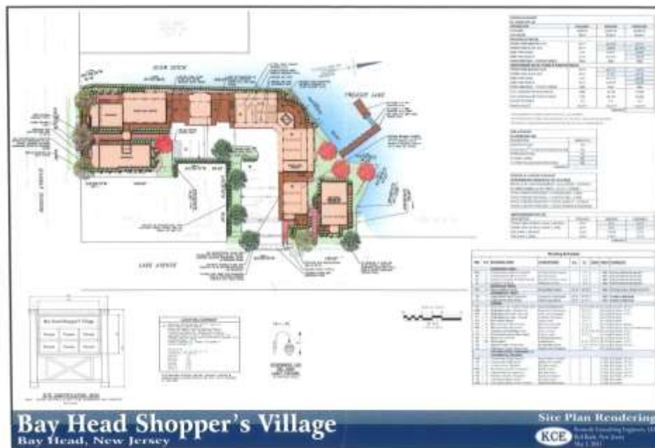
Figure 16: Plan Rendering of Shopper's Village – showing building layout, parking, and outdoor space
