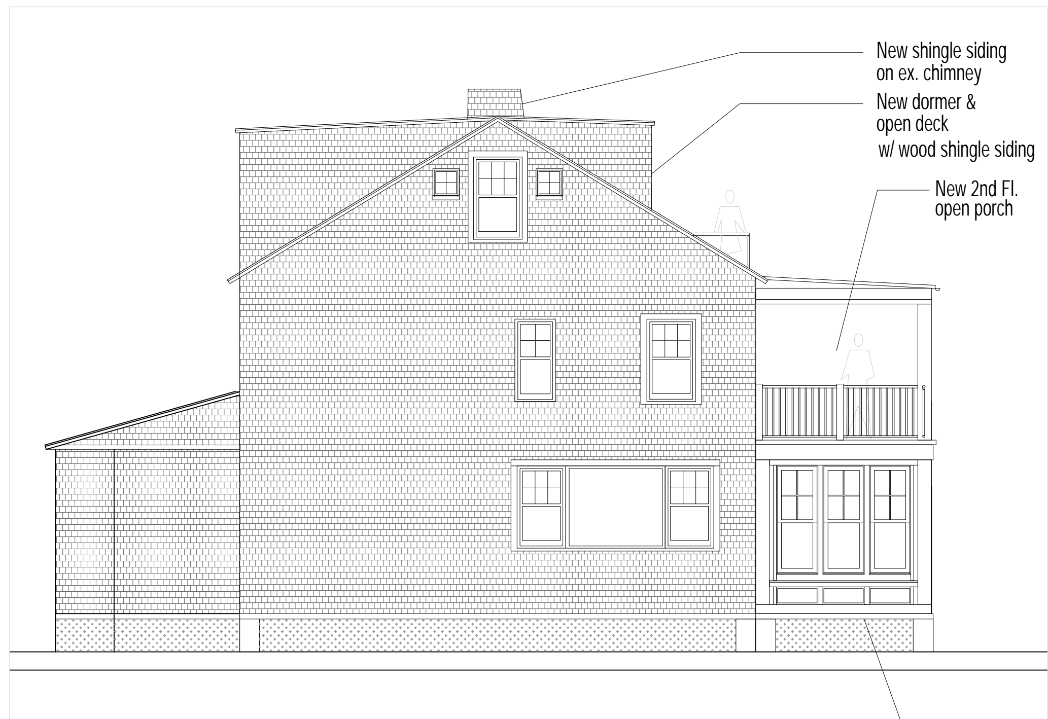
A4 2 PROPOSED WEST ELEVATION Scale: 3/16" = 1' - 0"
