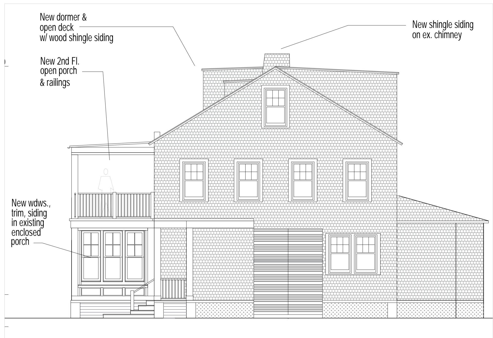
A4 4 PROPOSED EAST ELEVATION Scale: 3/16" = 1' - 0"
