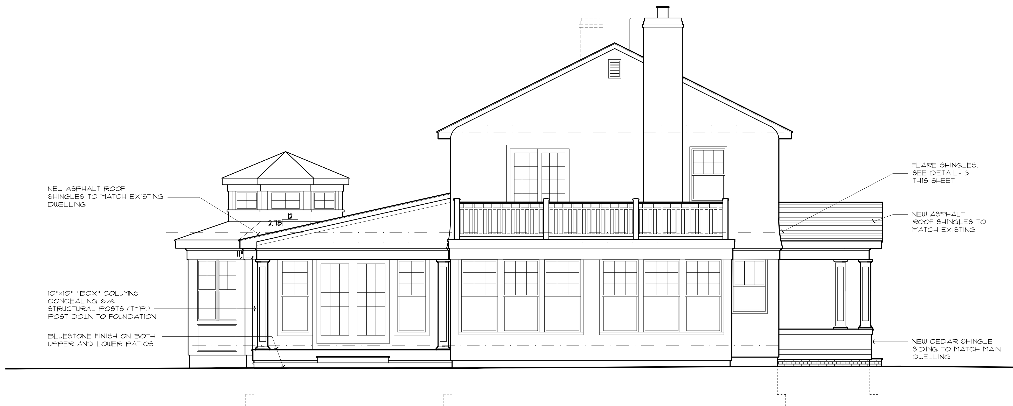
1 West Elevation SCALE: 1/4" = 1'-0"
